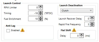
Note that these settings still need to be in accordance to engine fueling. You cannot just put any values in and expect the engine to perform properly. For spinning jou may need to run higher timing and less fuel enrichment to maintains power on the track.
